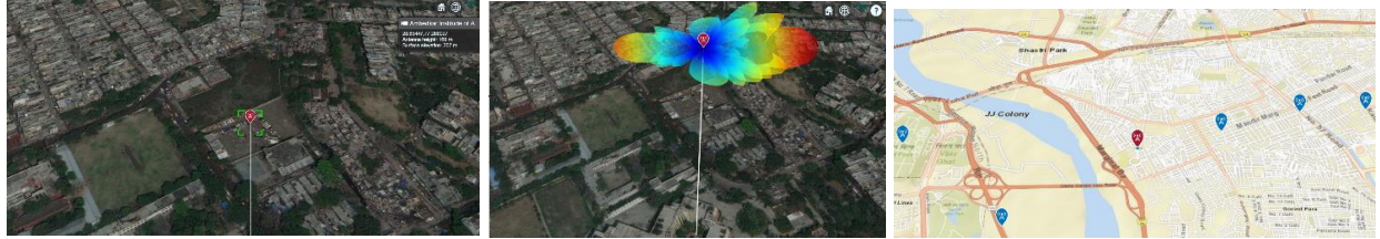
Figure 4: a) Showing the transmitter placed at Ambedkar Institute with height 169 meters b) Showing the radiation pattern at transmitter site c) Showing the receiver site location
